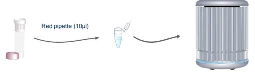
Take great care when setting up your positive control. The positive control template has the potential to give you a false positive signal in your other samples. Set positive controls up last after all other sample tubes are closed. Always change pipette tips between samples. You may even choose to set up positive controls in a separate room.
