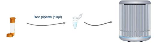
For every reaction to be run, use the red pipette to add 10µl of your EHV-1 reaction mix to every tube.
