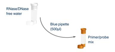
Then use the blue pipette to transfer 500µl of water into the brown tube labelled FluA\_M2\_v2.0 primer/probe mix. Cap and shake tube to mix. A thorough shake is essential to ensure that all components are resuspended. Failure to mix well can produce poor kit performance.
