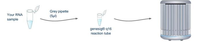
For each sample you wish to analyse, use the grey pipette to add 5µl of your RNA sample to the required reaction tube (already containing primer/probe mix and oasig® OneStep Master Mix). Close these tubes after adding the sample. Always change pipette tips between samples.
