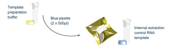
Use the blue pipette to transfer  $1000\mu$ I (2 x  $500\mu$ I) of template preparation buffer into the Internal Extraction Control RNA template tube. Cap and shake the tube to mix.
