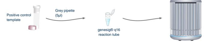
Take great care when setting up your positive control. The positive control template has the potential to give you a false positive signal in your other samples. Set positive controls up last after all other sample tubes are closed. Always change pipette tips between samples. You may even choose to set up positive controls in a separate room.
