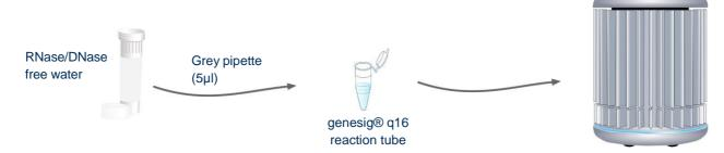
For each test you will require a negative control. Instead of RNA, water is used. The negative control sample should give a negative test result and thereby prove that any positive samples really are positive, and not tested positive due to contamination.
