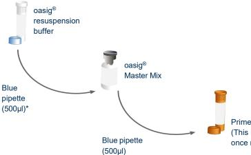
Use the blue pipette to transfer 500µl\* of the oasig® Master Mix resuspension buffer into the tube of lyophilised oasig® Master Mix and mix well by gently swirling. Then transfer all of that master mix into the brown tube labelled BFDV primers/probe.
