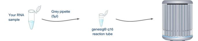
For each sample you wish to analyse, use the grey pipette to add 5µl of your RNA sample to the required reaction tube (already containing primer/probe mix and oasig<sup>®</sup> OneStep Master Mix). Close these tubes after adding the sample. Always change pipette tips between samples.
