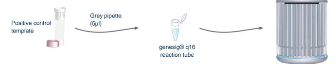
Take great care when setting up your positive control. The positive control template has the potential to give you a false positive signal in your other samples. Set positive controls up last after all other sample tubes are closed. Always change pipette tips between samples. You may even choose to set up positive controls in a separate room.
