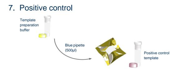
Use the blue pipette to transfer 500µl of template preparation buffer into the positive control template tube. Cap and shake tube to mix.
