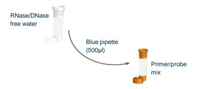
Then use the blue pipette to transfer 500µl of water into the brown tube labelled HIV2\_v2.0 primer/probe mix. Cap and shake tube to mix. A thorough shake is essential to ensure that all components are resuspended. Failure to mix well can produce poor kit performance.
