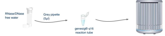
For each test you will require a negative control. Instead of RNA, water is used. The negative control sample should give a negative test result and thereby prove that any positive samples really are positive, and not tested positive due to contamination.
