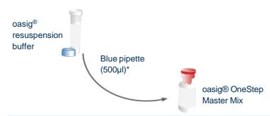
Use the blue pipette to transfer 500µl\* of the oasig<sup>®</sup> OneStep Master Mix resuspension buffer into the tube of lyophilised oasig<sup>®</sup> OneStep Master Mix and mix well by gently swirling.
