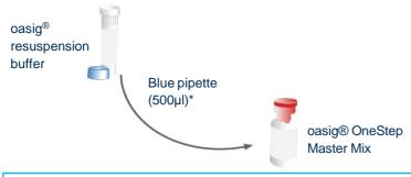
Use the blue pipette to transfer 500µI\* of the oasig® OneStep Master Mix resuspension buffer into the tube of lyophilised oasig® OneStep Master Mix and mix well by gently swirling.
