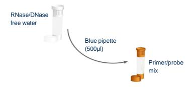
Then use the blue pipette to transfer 500µl of water into the brown tube labelled ISAV-HPR0 primer/probe mix. Cap and shake tube to mix. A thorough shake is essential to ensure that all components are resuspended. Failure to mix well can produce poor kit performance.
