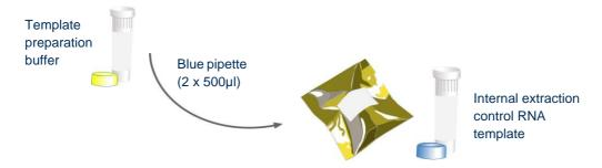
Use the blue pipette to transfer  $1000\mu$ I (2 x  $500\mu$ I) of template preparation buffer into the Internal Extraction Control RNA template tube. Cap and shake the tube to mix.
