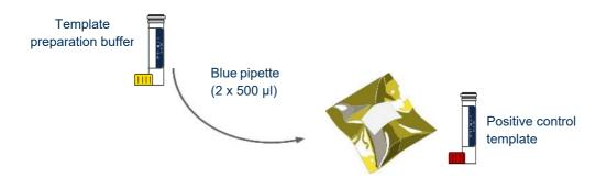
Use the blue pipette to transfer 1000  $\mu$ l (2 x 500  $\mu$ l) of template preparation buffer into the positive control template tube. Cap and shake tube to mix.
