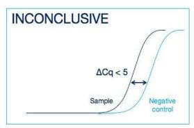
If the sample amplifies < 5 Cq earlier than the negative control, then the positive sample result is invalidated, and the result should be determined inconclusive due to test contamination. The test for this sample should be repeated.
