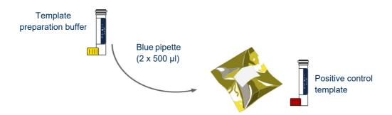
Use the blue pipette to transfer 1000  $\mu$ l (2 x 500  $\mu$ l) of template preparation buffer into the positive control template tube. Cap and shake tube to mix.
