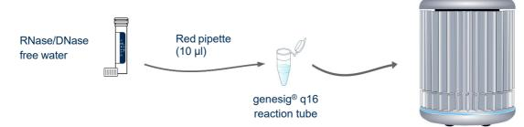
For each test you will require a negative control. Instead of DNA, water is used. The negative control sample should give a negative test result and thereby prove that any positive samples really are positive, and not tested positive due to contamination.
