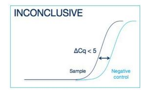
If the sample amplifies < 5 Cq earlier than the negative control, then the positive sample result is invalidated, and the result should be determined inconclusive due to test contamination. The test for this sample should be repeated.
