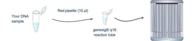
For each sample you wish to analyse, use the grey pipette to add 10  $\mu$ l of your DNA sample to the required reaction tube (already containing primer/probe mix and oasig<sup>®</sup> Lyophilised 2X qPCR Master Mix). Close these tubes after adding the sample. Always change pipette tips between samples.
