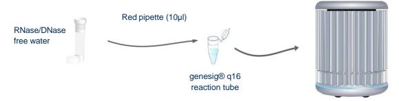
For each test you will require a negative control. Instead of DNA, water is used. The negative control sample should give a negative test result and thereby prove that any positive samples really are positive, and not tested positive due to contamination.
