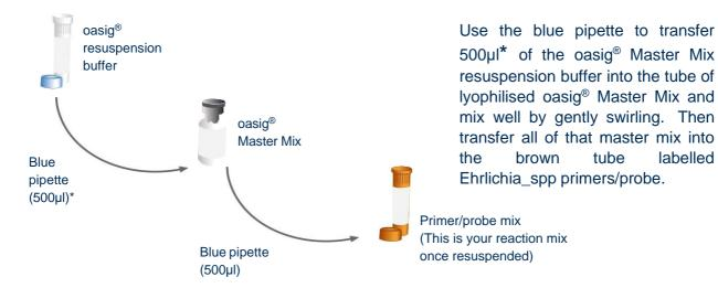
\*Transferring 525µl of the oasig® Master Mix resuspension buffer to your oasig® Master Mix (instead of the 500µl recommended above) will enable you to take full advantage of the 50 reactions by accounting for volume losses during pipetting. In order to do so with the genesig® Easy fixed volume pipettes use 1x blue, 2x red and 1x grey pipettes to make the total volume. Please be assured that this will not adversely affect the efficiency of the test.
